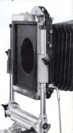
Critical focusing on the groundglass with wide-angle bellows used as focusing hood and attached focusing magnifier, excluding all extraneous light.
