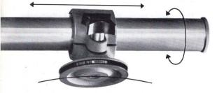
Tripod head with large seating area, hollowed in the middle. Socket accepts long tripod screw. Easy movement on extensible optical bench. Bench centered swiveling of entire camera. Screw-in extensions of optical bench are rigidly fixed without joints.
