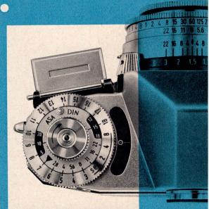
On the CONTAFLEX II the meter shows aperture and shutter speed, on the CONTAFLEX IV the exposure-value, because the models III and IV have exposure-value shutters with coupled shutter speed and aperture settings. These shutters also have a lock to prevent accidental alteration of the flash setting lever.
