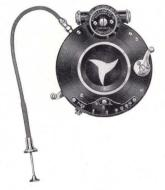
ments are met by a between-lens shutter. An ingenious locking device prevents the making of instantaneous bulb or time exposures unless desired The steel segments of the shutter leaves form a star-shaped opening giving even illumination during the whole exposure, while an independent diaphragm is provided.
