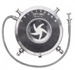
revolve in making the exposure. The leaves when opening and closing assume a star-shaped aperture, thereby giving the greatest possible illumination to the plate. Besides bulb and time exposures, it has a range of from one second to 1-300th part of a second, the latter being sufficiently fast to cover the utmost emergency; it works quietly and does not jar.
