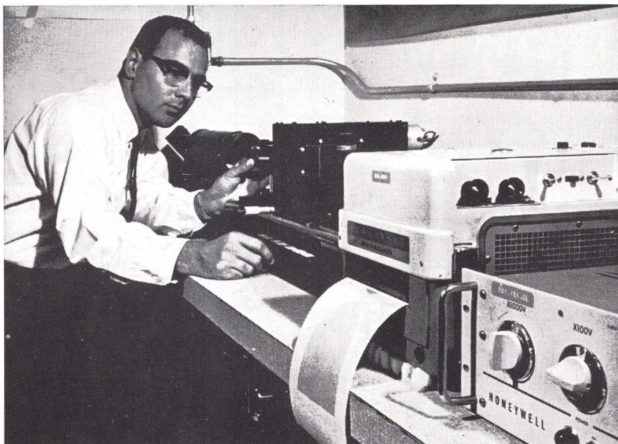
Honeywell testing for image fidelity of lenses includes this sophisticated checkout on a Honeywell Visicorder Oscillograph.
