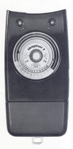
**IKOPHOT CD** A new CdS Exposure Meter that has high measuring accuracy even under extreme lighting conditions. The jeweled bearings and temperature compensated cadmium sulfide photocell has a range of 20 light values and the film-speed scale ranges from 6 to 3200 ASA. Exposure times range from 1/1000 sec. to 1 hour and lens apertures from f/1 to f/45. The Ikophot CD includes a built-in diffuser for incident light readings. Price: \$34.95 with case
