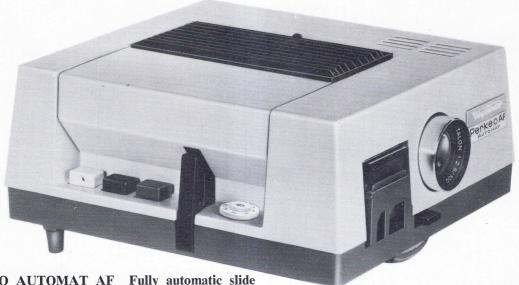
**PERKEO AUTOMAT AF Fully automatic slide projector.** This 2" x 2" slide projector focuses automatically and is remote control operated — forward, reverse, timer. It has an extra bright Halogen lamp 24 volts/150 watts with fan and special lamp-saving switch. The automatic timer sets at 5 to 30 seconds. The AF has an aspherical condenser system and adjustable voltage selector of 120/240 volts.
