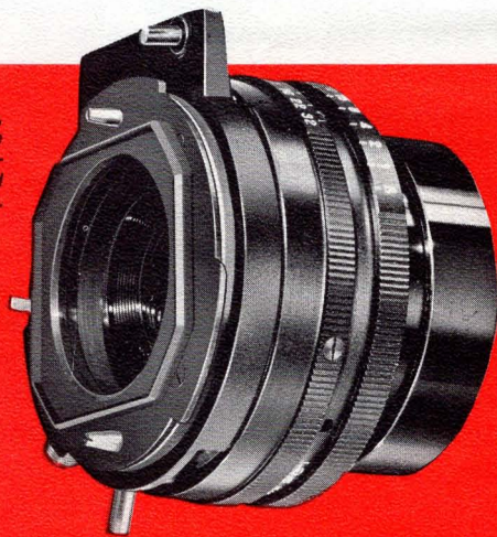
Lenses lock on solidly, detach readily, couple automatically to range-finder, focus knob and shutter cocking action.
