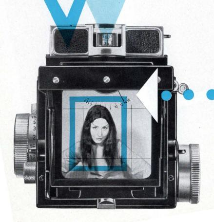
The powerfully brilliant finder image, produced by the Fresnel-type field lens combined with the ground glass screen, is an important feature of all lkoflex models. The finder of this 2½ × 2½-inch twin-lens reflex camera shows, however, not only a view of the subject; it exactly indicates also the sharpness of the image, and the reading of the built-in Zeiss Ikon photo-electric exposure meter. At a glance into the viewfinder hood you see everything
