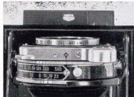
Figures on lens and shutter mounts, visible from above, show distance focused, depth of field, diaphragm stop and shutter speed.
