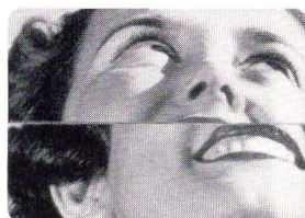
The halves of the image, as seen through the range finder, are split and out of alignment here as the lens is focused for a distance greater than that from camera to subject.
