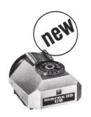
Measuring angle = angle of view! The CdS exposure meter built into this prism finder attachment gives exact measurement through all interchangeable lenses, even for close-ups. Operation is very simple: set preselected shutter speed, depress button and turn aperture setting ring on camera until the pointer in the finder is zeroed on a mark - and you are ready to shoot. The range of measurement is considerable: the lower limit for 100 ASA and f 8 is 4 sec.
