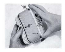
Press (8) the rapid sequence lever (J) on the front of the IKONETTE two or three times until the upper row of perforations engages the sprocket (9).
