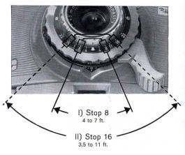
Keep in mind: The smaller the aperture the greater the depth of field and vice versa.
