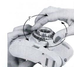
Turn ring (F) until the red mark is opposite the shutter speed required, (Figures stand for fractions of a second, e. g.  $25 = \frac{1}{25}$  second.) "B" is for time exposures, the shutter remaining open as long as lever is pressed down.
