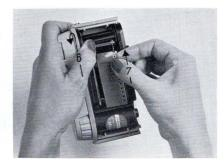
Insert film cartridge. If prong (5) does not fit neatly into the cartridge, turn rewind knob (N) a little (4).
