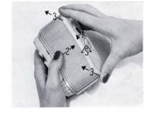
Turn the locking bar (S) to the red dot (1). Push down the back (2) with your thumb and lift it off (3).
