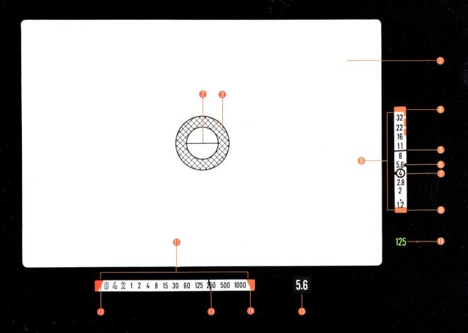
You can tell at a glance which mode you are in by the position of the information display. On manual and shutter-priority AE it is on the right. With the AE Finder FN installed and set for aperture-priority AE, the display appears below the image.
