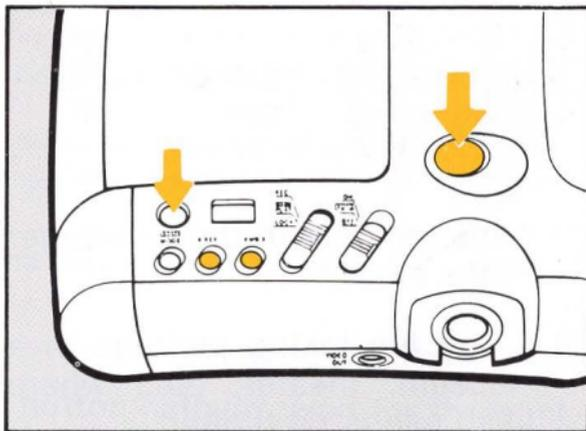
The exposure compensation button applies approximately +1.5 step compensation.
