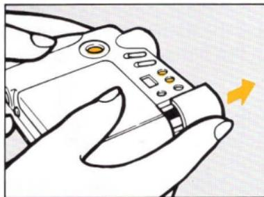
3. Insert a fully-charged battery in the direction of the arrow.
