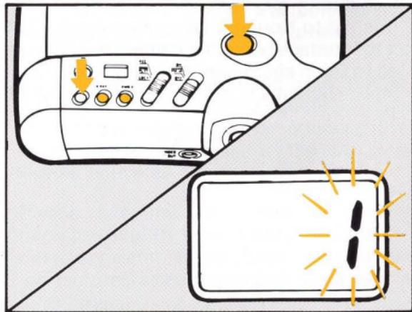
The picture disappears from the screen and the track number in the display panel blinks twice. The picture is erased then.
