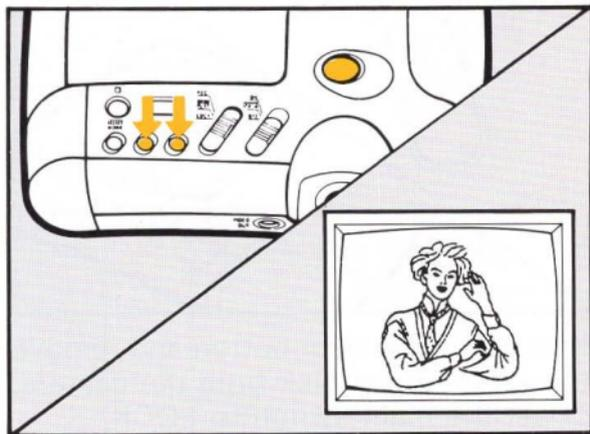
The screen shows the next picture each time you press the forward or reverse-feed button. Pictures keep changing (4 pictures fed per second) when you hold the button down.
