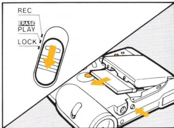
Press the disk eject button and remove the video floppy disk from the camera, or set the main switch to LOCK.
