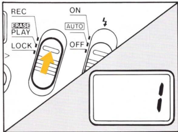
Track number "1" appears in the display panel and the picture recorded in the first track of the disk is shown on the TV screen.
