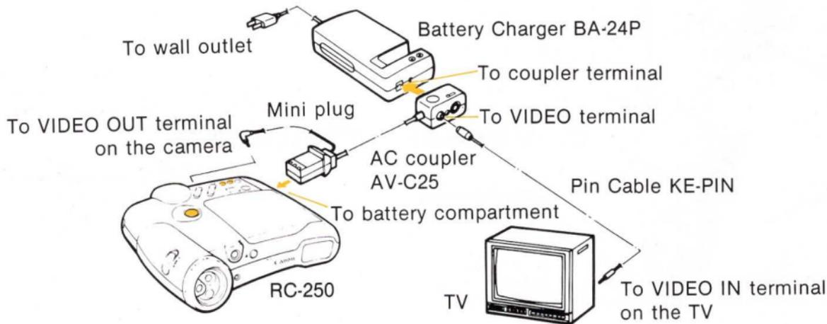
1. Connect the VIDEO terminal on the AC Coupler AV-C25 (battery charger side) and the VIDEO IN terminal on the TV with the Pin Cable KE-PIN.
