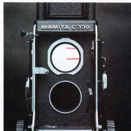
The shutter plate (behind the taking lens) is in the down position
