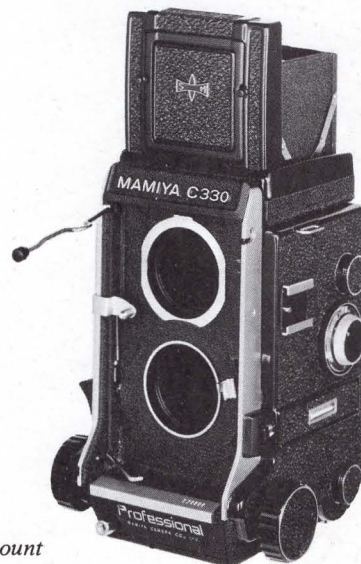
The shutter plate (behind the taking lens) is in the down position
