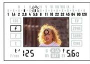
Measuring Flash: In backlit scenes when using fill in flash, it is vital to measure the value of the flash and the value of the ambient portion of the light available. The ULTRA-SPOT 2 does this involved procedure instantaneously. When we meter the main part of the subject (the face), the ULTRA-SPOT 2 displays the resulting exposure in digital form (f5.6) and also on the analog scale as a flashing cursor. The ambient light is displayed on the analog scale as a constant cursor.
