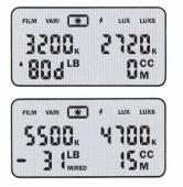
Filters can be displayed as mired values or as Kodak Wratten™ types. For fluorescent light, the required color compensating filters are indicated as CC values.
