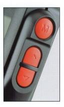
Just press a button: The button for measuring the light is conveniently placed on the right side of the meter, as are the buttons for changing the values up or down. Buttons for changing the functions left or right are on the front of the meter.
