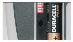
The functions center: The DIP switches are placed beside the battery in the compartment.
