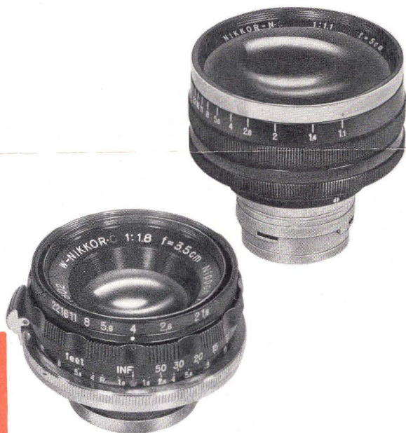
NIKKOR 50mm f1.1—New ultra high speed lens. 9 elements in a light weight mount. 'Click stop' settings.
