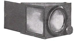
Certain reproduction processes demand reversed negatives to avoid stripping the film. This reversal is obtained in the negative by placing a right angle prism on the lens, usually at the front. No lens can work to any higher accuracy than the prism with which it is used.
