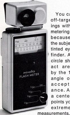
You can't get off-target readings with the spot metering attachment because you sight the subject through a tinted eyelevel viewfinder. A bright-line circle shows the exact area covered by the 10° angle of acceptance. And a center spot pinpoints your target for extremely critical
