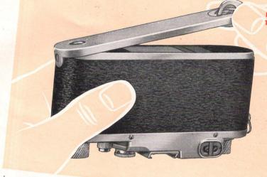
8. Hook the baseplate over the pin, close it and turn the locking handle to "CLOSED" (or ZU). The camera is now light-tight.
