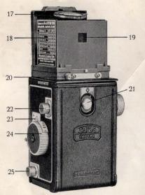
The ZEISS IKON IKOFLEX II is a twin-lens mirror reflex camera with a ground glass viewfinder rendering brilliant pre-views of the object. The Jkoflex II is made for picture sizes of  $2^1/4'' \times 2^1/4''$ . It is equipped with a J-coated, well-corrected Zeiss Jessar f/3.5 focal length 3 ins. as well as a viewing lens with equal speed and focal length, a Compur shutter with flashlight synchronization, automatic film stop with double-exposure prevention and frame counter
