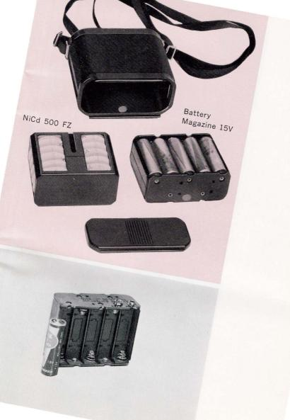
**2** Remove the bottom cover of the Battery Case by sliding it either to left or right. Facing the battery contacts upwards, load NiCd Battery 500 FZ properly by matching the groove on the 500 FZ and the guide line inside the Battery Case, and replace the bottom cover
