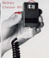
**3** Plug the cord of the Battery Connector into the socket situated at the bottom of the Motor Drive Unit. The plug-in position is set by the matching groove.
