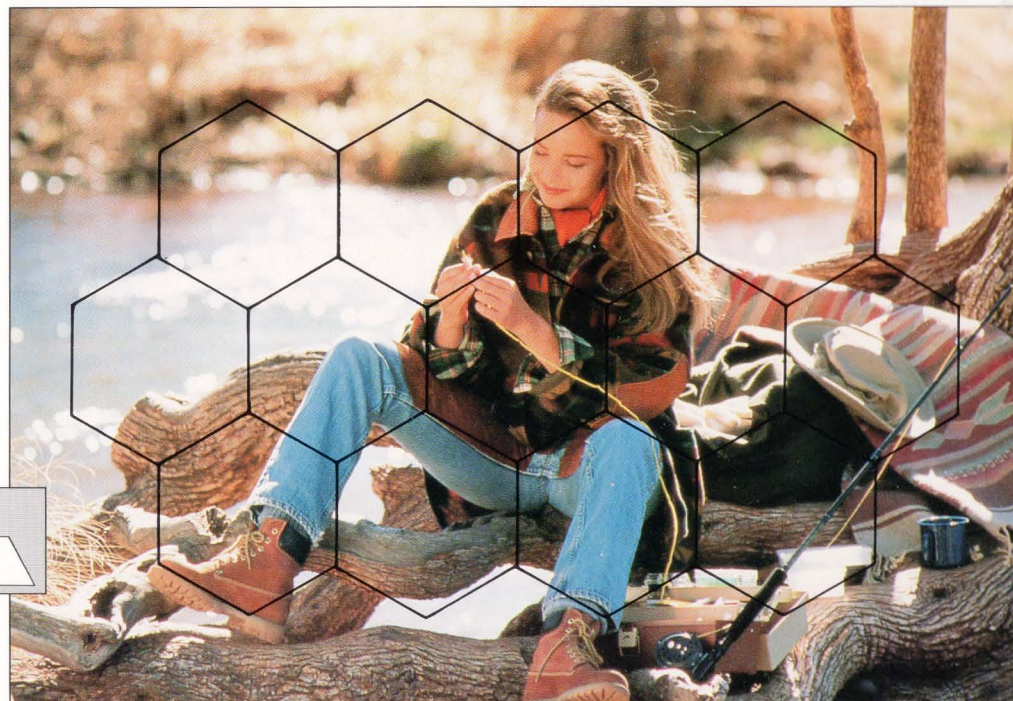
14-segment Honeycomb-Pattern Metering measures image brightness in 13 sections, plus the background, for optimum exposure.
