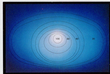
The Center-Weighted pattern of the MX. Figures denote percentage of importance placed upon area by the GPD's.
