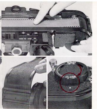
7 Put this take-up magazine into the take-up magazine chamber in the same manner as the supply magazine was inserted, and push in the magazine attachment knob.
