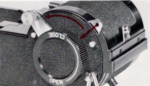
**3** Align the back cover grooves of the camera with the rails of the Film Chamber Then push in the camera until the index lines of the camera and the white dots of the Film Chamber match.
