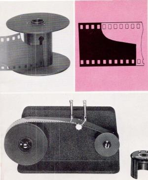
2 Wind a strip film to a spool of the magazine by using Film Loader 250 in a darkroom. Insert a strip film either directly into the supplyside shaft of the Film Loader or by using the spool attached to the Film Loader Raise two film holding rollers.
