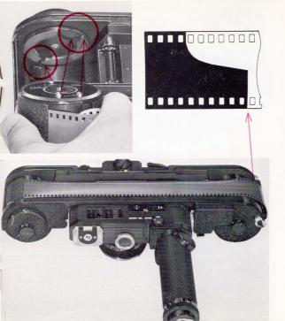
**3** Load a magazine, containing unexposed film, in the supply magazine chamber Fit the two projections and the release button on the top side of the magazine to the notch on the upper part of the magazine chamber Push in the magazine attachment knob.
