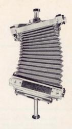
Horizontal Swing Both front and back of the camera can be swung 12 degrees in either direction on a vertical axis for horizontal distortion correction. This adjustment is helpful in correcting diverging lines and increasing depth of focus.
