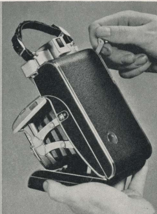
One operation sets shutter, actuates window cover, advances film.
