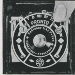
Setting the built-in self timer on the f.4.5 Kodak Vollendia
