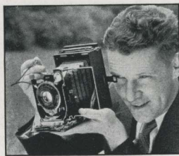
The wire-frame direct-view finder is particularly valuable in "following" moving subjects
