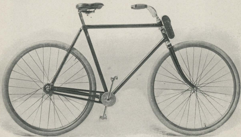
NO. 2 FOLDING POCKET KODAK BICYCLE CASE ATTACHED TO HEAD OF MACHINE BY MEANS OF CLAMP.
