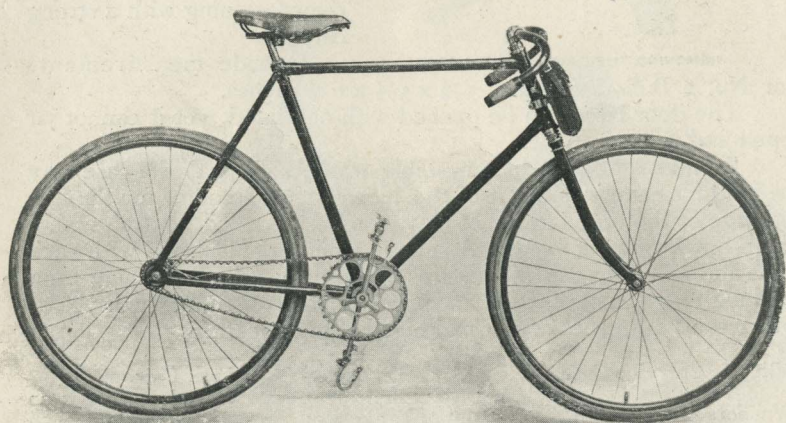
FOLDING POCKET KODAK BICYCLE CASE ATTACHED TO HEAD OF MACHINE BY MEANS OF CLAMP.
