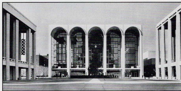
Lens shifted vertically, camera level, verticals remain parallel.
