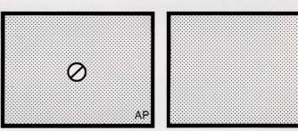
**Type AP:** Central diagonally-oriented split-image focusing screen with surrounding Acute Matte field. It provides an unusually bright image with f/5.6 or faster lenses.
