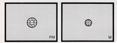
**Type PM:** Standard Acute Matte Focusing Screen supplied with XD cameras has both split-image rangefinder and surrounding microprism collar.
