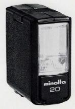
Type: Clip-on manual electronic flash for cordless hot-shoe operation 2 AA-size AM or C-Zn cells 33 with ASA 25 film Power Source: Guide Number: Recycling Time: 9 sec. with fresh batteries; ready lamp comes on when recycling is complete Synch Contact: Wired for hot-shoe operation; open-flash button Flash Duration: 1/2000 sec.
