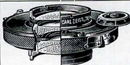
Standard Mount N for Travelling and large Stand Cameras with bellows extension.
