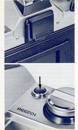
To prevent stray light from entering the viewfinder from the rear and possibly affecting the meter reading, it is a good idea to cover the eyepiece with the viewfinder cover which is inserted into the accessory shoe. This cover can be attached to the holder on the viewfinder eyepiece. After doing so, press the shutter button.
