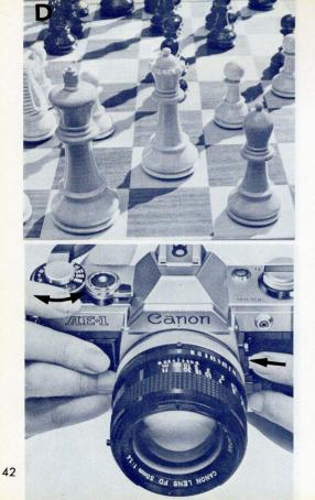
2 Effects of Changing the Aperture Because this camera is an AE camera with shutter speed priority, when you change the shutter speed, the aperture will also change. If you change the speed by one gradation, the aperture also changes the equivalent of one gradation. Aperture changes have an effect on the photographic expression as follows:
