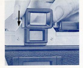
Accessories such as an eyecup, dioptric adjustment lenses, angle finders, and magnifier can be attached to the viewfinder eyepiece.
