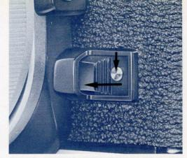
be done after advancing the film. If the film is not advanced, the stopping-down of the lens diaphragm would only be possible down to the aperture of the previous exposure. Also, when the aperture ring is set at the "A" mark, the stopped-down lever cannot be pressed in. Please note that stopped-down metering is impossible when the FD lens is mounted on the AE-1.
