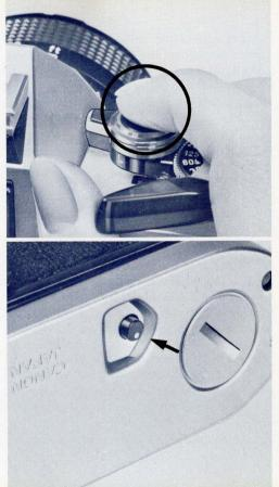
To rewind the film, press in the small rewind button on the bottom of the camera, unfold the rewind crank and turn it in the direction of the arrow on top of the rewind crank. When the frame counter has reached the "S" mark, you should stop rewinding. Then pull up the rewind knob to open the camera back and lift the cartridge out.
