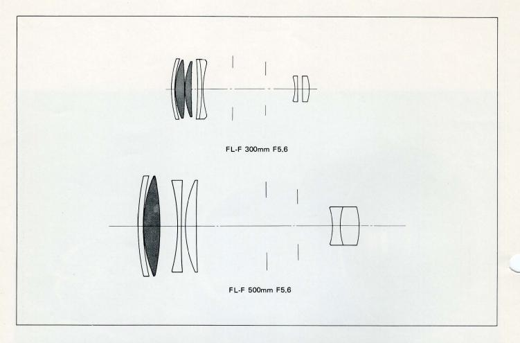
Canon, through its vast technological resources, has succeeded in manufacturing large-size artificial fluorite (CaF<sub>2</sub>) crystals for the commercial production of apochromatic lenses. This technical break-through promises a new future in the further development of telephoto and high magnification zoom lenses.
