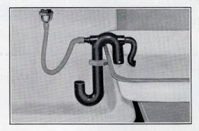
THE Eastman Automatic Tray Siphon is an inexpensive device that converts an ordinary tray into a very effective washing machine. It was invented by a scientist and it works on correct scientific principles—puts fresh water in at the top and siphons out the chemically laden water from the bottom of the tray.
