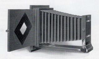
AVERY practical enlarging camera with revolving negative carrier, and rising and falling front which makes it easy to adjust the image on the paper easel. A rack and pinion with large knob simplifies focusing. The carrier is fitted with nested kits down to  $3\frac{1}{4}$  x  $4\frac{1}{4}$ , the front board is  $5\frac{1}{2}$  x  $5\frac{1}{2}$  inches and the bellows draw, 22 inches.
