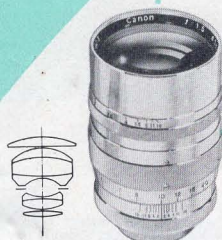
CANON 85mm f:1.5 Semi-Long-Focus Lens • 7 elements Angle of View: 29° Apertures: f:1.5 to f:16 Focuses: from 3.5 feet
