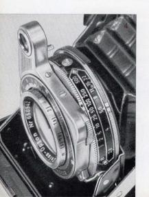
catch of the ZEISS IKON cable release. The shutter is set by lever (17). Except for  $^{1}/_{500}$  sec. it does not make any difference whether the exposure time is set before or after setting of the shutter. With the  $^{1}/_{500}$  sec. setting the exposure time must be set before the shutter is wound.
